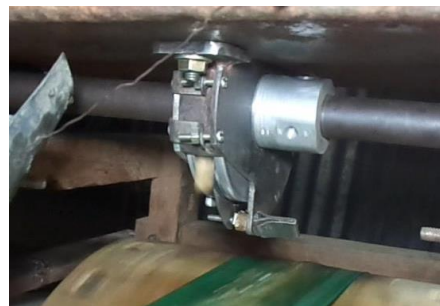
Fig. 4. Seed knocked out of cell by positive seed knocking device
