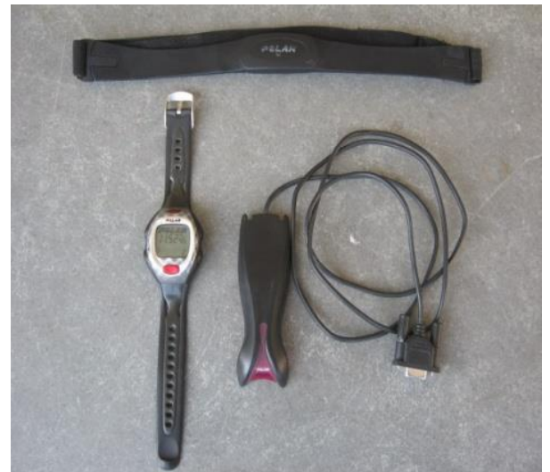
Figure 1. Heart rate monitor (transmitter, receiver and interface) (Polar electro, Finland)
