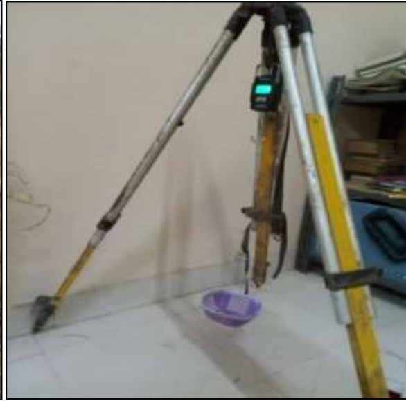
Figure 2. Instrumentation designed for measurement of root tensile strength
