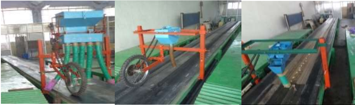
(a) Cell type (b) Spoon type (c) Cup type Figure 1. Metering mechanisms with metering boxes on sticky belt test set-up
