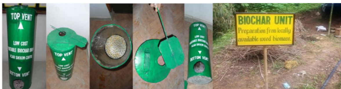
Figure 1. Preparation of biochar by low cost portable drum (kiln)
