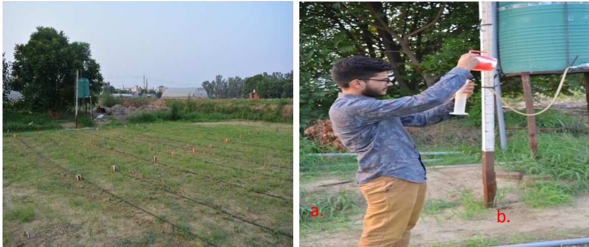
Figure 1. A view of the installed low head drip irrigation system and measurement of emitter discharge.
