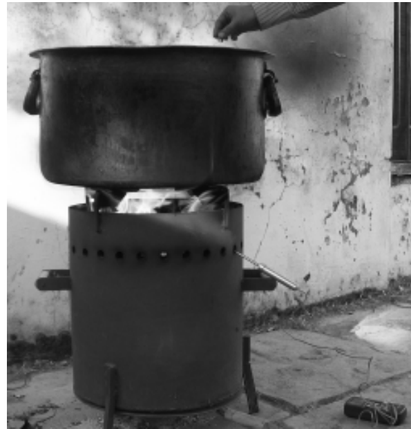
Fig. 3: Turmeric Curing with Biomass combustor
