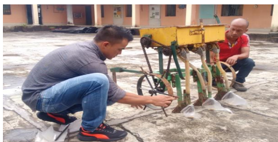
Figure 2. Calibration of power tiller drawn seed drill (Maize variety used: RCM 76)
