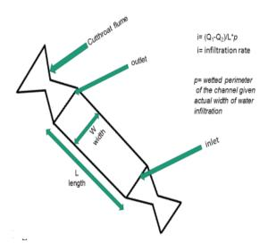
The infiltration is given by the difference of discharges between the inflow and outflow flume divided by the actual area of infiltration which is the product of length of uniform channel section and the wetted perimeter of the channel. The measurement of wetted perimeter is taken very carefully by taking average value of multiple measurements within the channel section.
