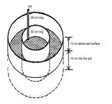
Figure 1. Schematic Diagram of Double Ring Infiltrometer
